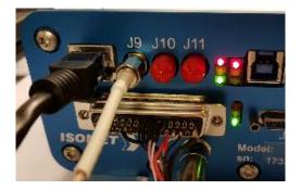
It is recommended that USB or Ethernet are connected to the iMS4- prior to power up. We recommend attempting USB communication AFTER initialization is complete.
