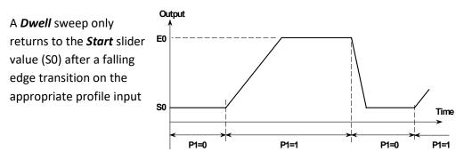
Both plots show a ramp on output J2, controlled using input P1
